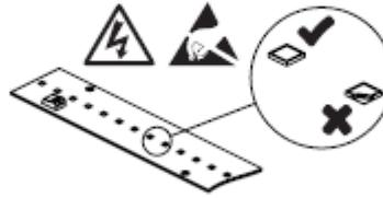
Acceptable luminaire with or without ZHAGA socket mounting angle relative to the ground.
